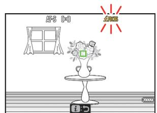
**5 Press the button you intend to use for recall of the focus position saved in Step 4.**
