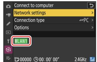
A wireless connection has now been established between the camera and the computer.
