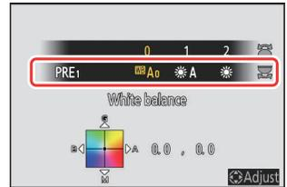
Options for the selected setting, if any, can be selected by holding the **WB** button and rotating the sub-command dial.
