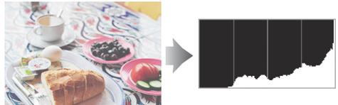
Increasing exposure compensation shifts the distribution of tones to the right, while decreasing exposure compensation shifts the distribution to the left. Histograms can provide a rough idea of overall exposure when bright ambient lighting makes it difficult to see pictures in the monitor.
