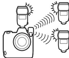
\* Radio flash control is available only when a WR-R11a or WR-R10 is connected to the camera.
