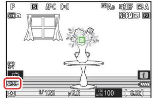
**2** Keeping the center of the sub-selector pressed, recompose the photograph and shoot.
