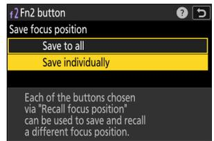
4 Focus on the desired subject in the shooting display and press and hold the control to which [Save focus position] is assigned.
