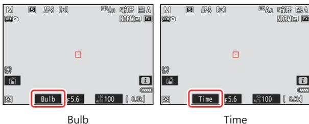
Note that the exposure indicators are not displayed at a shutter speed of **Bulb** or **Time**.
