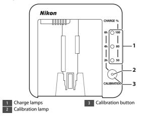
If the calibration lamp flashes when a battery is inserted, the battery needs to be calibrated.
