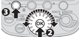
**3** Repeat Step **2** to select all desired items, then press Function button 1 [BACK] to return to set-up mode.
