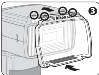
**3** Place the filter holder on the flash head with the Nikon logo facing up, as shown in the diagram, and insert into the slit at the top.
