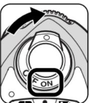
2 Turn the SB-400 and the camera body on.
