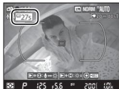
Matrix metering is used regardless of the metering method selected. The camera adjusts shutter speed and ISO sensitivity automatically.
