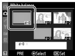
To use the new value for white balance, select preset d-0 (if no value has been measured for white balance before d-0 is selected, white balance will be set to a color temperature of 5,200 K, the same as **Direct sunlight**). The new white balance value will remain in preset d-0 until white balance is measured again. By copying preset d-0 to one of the other presets before measuring a new value for white balance, up to five white balance values can be stored (147).
