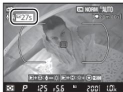
During live view, the camera displays the shutter speed and aperture in effect at the start of live view. Exposure is metered again when the shutter-release button is pressed all the way down.
