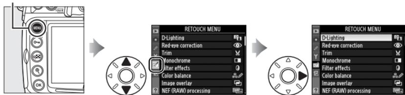
The options in the retouch menu are used to create trimmed, or retouched copies of existing pictures. The retouch menu is only displayed when a memory card containing photographs is inserted in the camera.
