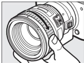
If the lens supports autofocus with manual override, after focusing using autofocus you can keep the shutter-release button pressed halfway and rotate the lens focus ring to fine-tune focus manually. To refocus using autofocus, press the shutter-release button halfway again.
