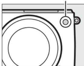
The AF-assist illuminator will not light to assist the focus operation in advanced movie mode, during movie recording, or when **Off** is selected. If the AF-assist illuminator does not light, autofocus may not produce the desired results when lighting is poor.
