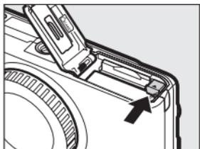
To remove a memory card, first press the card in to eject it (①); the card can then be removed by hand (②).
